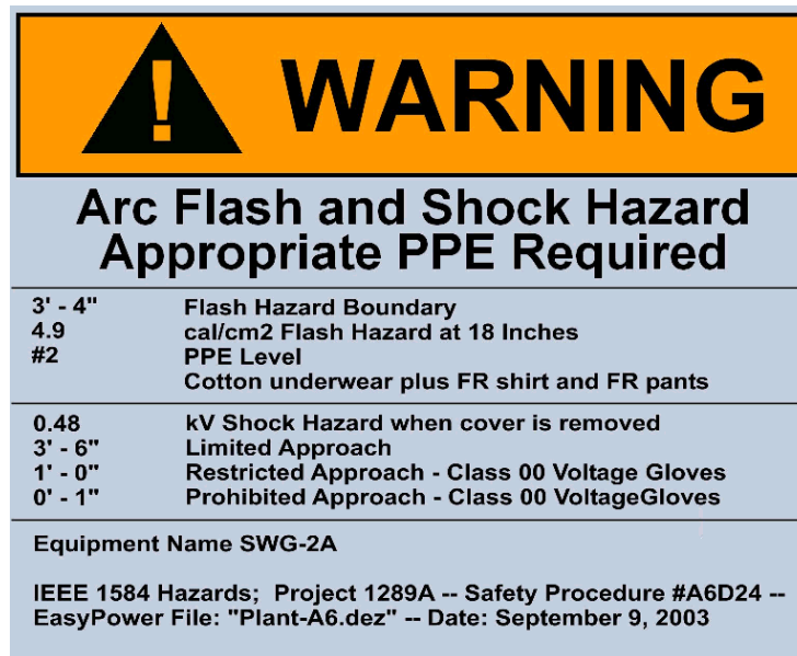
Figure 4.5: Example of arc flash warning label printed from EasyPower
