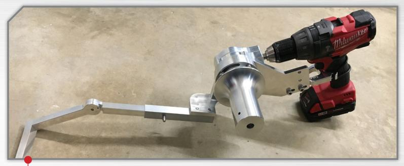
The CP1000 measures only 24" long when fully extended. When collapsed it easily fits into a tool bag. The heavy-duty drill chuck and handle lock attachment provide a sturdy base of operation. Wires up to 1/0 gauge can be pulled using the device.
