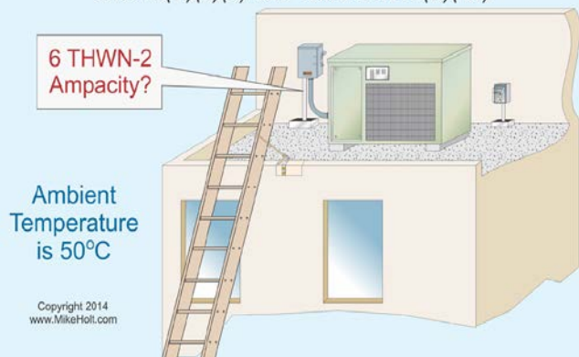
Conductor Ampacity - Ambient Temperature Correction 310.15(B)(2)(a) and Table 310.15(B)(16)
