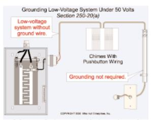
FIGURE 5-4 Safety grounding is not required for the metal parts of equipment and metal raceways for systems operating at less than 50 volts.
