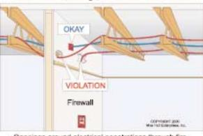
Openings around electrical penetrations through fireresistant rated walls, partitions, floors, or ceilings are required to be firestopped using approved methods to maintain the fire resistance rating.
