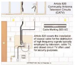
Coaxial cables are not required to be installed in raceways.
