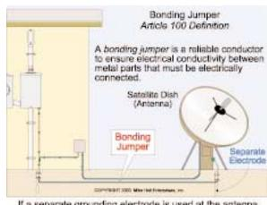
If a separate grounding electrode is used at the antenna, a bonding jumper run to the power grounding electrode system is required, See Section 810-21(j). tion equivalent to the wall of the equipment.
