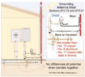
The metal structure (mast) supporting HAM, television, and satellite receiving antennas must be bonded to the building grounding electrode system.
