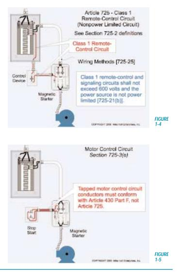
Author's Comment: Motor control circuit conductors tapped from the load side of a motor's short-circuit and ground-fault protective device are not considered a Class 1 remote-control circuit [725-3(e)]. The motor control tap conductors must be installed in accordance with the
