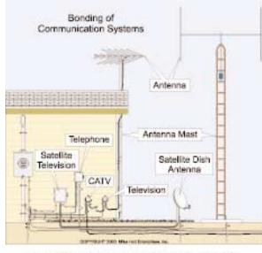
Metal parts of communications systems must be bonded to the building grounding electrode system. FIGURE 5-7 buried in the earth must be listed for direct burial and marked "DB" [800-40(c), 820-40(c), and 830-40(c)].
