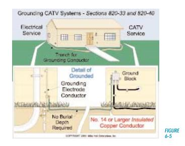
No.14 or larger insulated copper conductor run in as straight a line as practicable [820-40(a)], **Fig. 6-6**.
