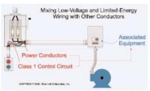
Class 1 control circuits and power conductors associated with the same equipment can occupy the same raceway, but Class 1 circuits cannot occupy the same cable, enclosure, or raceway with other low-voltage or limitedenergy circuits.
