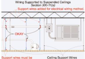
Support wires must be secured at both ends.
