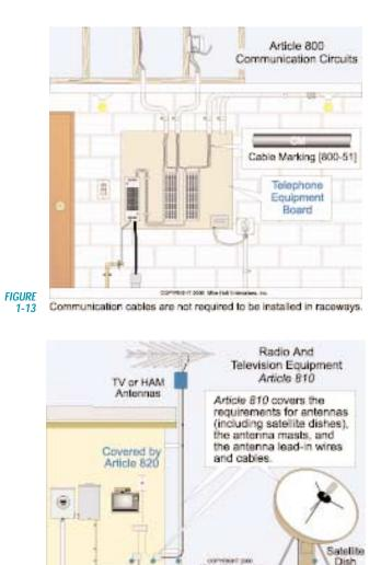
[800-50 and 800-511. Cables that meet this requirement are marked CM (Communications) or MP (Multipurpose). Optical fiber cables used for telecommunications circuits must be installed in compliance with the requirements of Article 770 [800-52(a)(1)].
