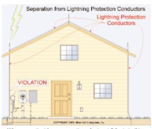
FIGURE 7-16 Where practicable, a separation of a least 6 feet shall be maintained between communication cables and lightning protection conductors.
