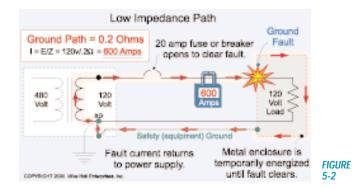
grounded conductor (neutral) resulting in a low ground-fault return path, **Fig. 5-2.**
