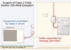
Class 2 control cables can be supported by the raceway that supplies power to the equipment controlled by the Class 2 cable. FIGURE 7-21 Author's Comment: Section 300-11(a) does not permit electrical wiring to be secured to ceiling support wires, but it does permit independent support wires secured at both ends to be used for the support of electrical wiring. Technically this rule does not apply to low-voltage or limited-energy cables because
