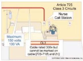
Class 3 circuits over 30 volts can have higher power capacity (100 VA) than Class 2 circuits (0.5 VA).
