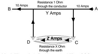
Figure 15. Parallel Path Through A Conductor And Flow Of Current Through The Earth with Variable Resistance Values
