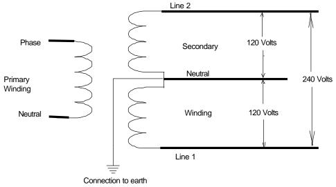
Figure 12. Phase to Neutral Primary Connection with Secondary winding Center Tapped
