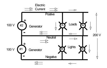
Figure 5. 3-Wire Direct Current Electrical System Conductor Used as Current Return Path
