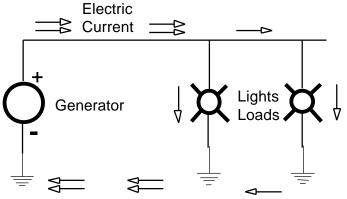
Figure 4. Direct Current Electrical System Earth Used as Current Return Path
