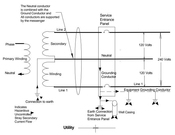
Figure. Conflict between the NESC and the NEC over the Grounding of the Neutral.
