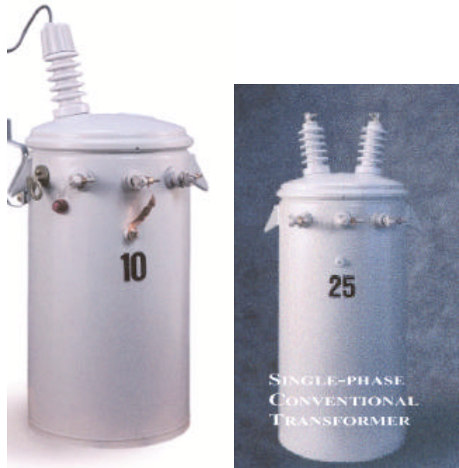
Figure 21. Left – Single Bushing Transformer With Ground Strap Connecting Secondary Neutral To Metal Can Of Transformer (Shown just above the “10”), Which Is the Primary Connection. Right – Two Bushing Transformer.
