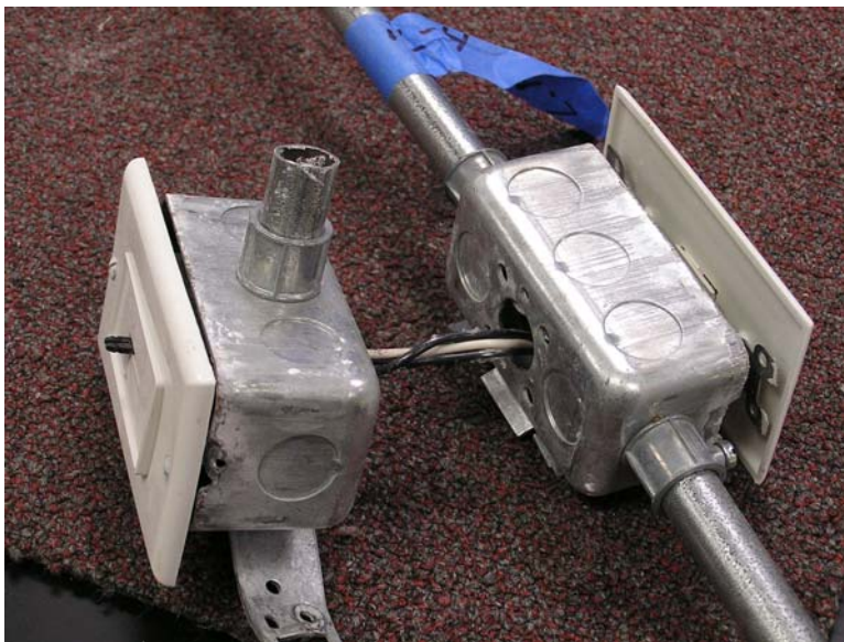
Fig. 33 – House IL-4, Open Conductors In Wall Between Boxes
