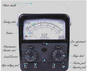
Now terminate one lead of an analog ohmmeter to the intersystem bonding terminal, the grounding electrode conductor, or the ground bar within service disconnect, then contact the other lead to the metal parts of pool motor, heat pump, salt chlorinator, pool junction box, pool light, hand rails, ladders, and any parts within five feet of the pool water.
