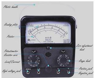
Now terminate one lead of an analog ohmmeter to the intersystem bonding terminal, the grounding electrode conductor, or the ground bar within service disconnect, then touch the other lead to the metal parts of pool motor, heat pump, salt chlorinator, pool panel, pool junction box, and pool light.
