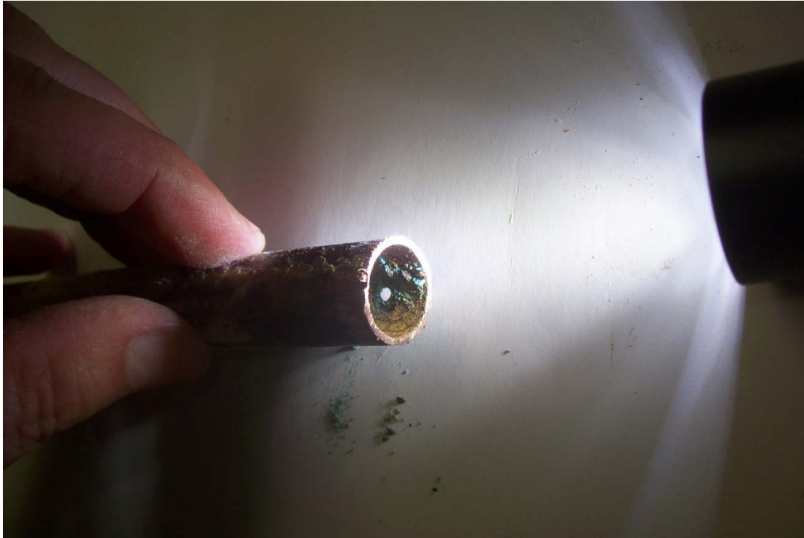
Figure (H2f): A view of a similar pinhole looking from the inside.
