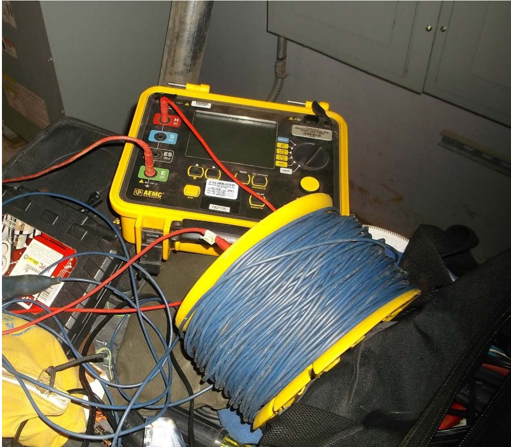
Figure (T1d): A fall of potential test was also done to test the earth triad. The test results in the report appeared to be within specification.
