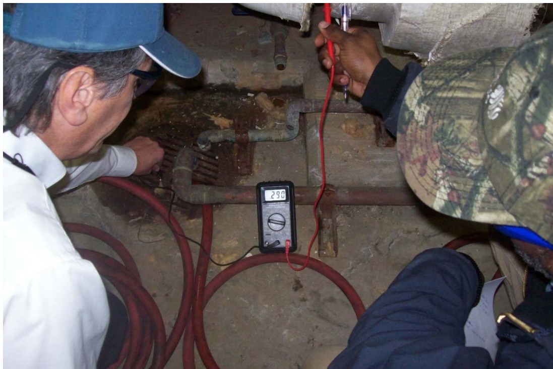
Figure (H1c): A view of another test on another day. With an Omega volt ohm meter, we measured 0.29 volts DC from pipe to wet floor drain grate (earth ground).
