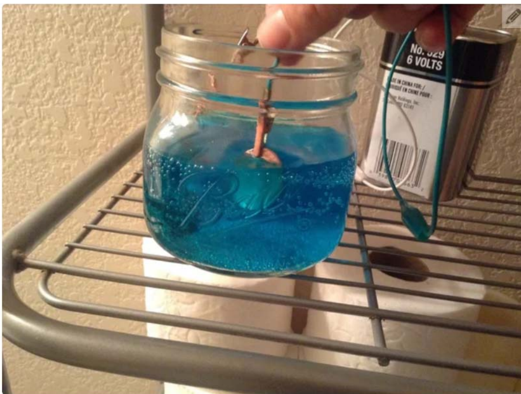
Figure (S2a): A view of the coin plating in action. A copper pot scrubber is used as the donor. The quarter is the recipient. A dry cell 6 volt DC battery is the driver. Note that AC (Alternating Current) will not cause metal transfer (AC will not cause pinholes).
