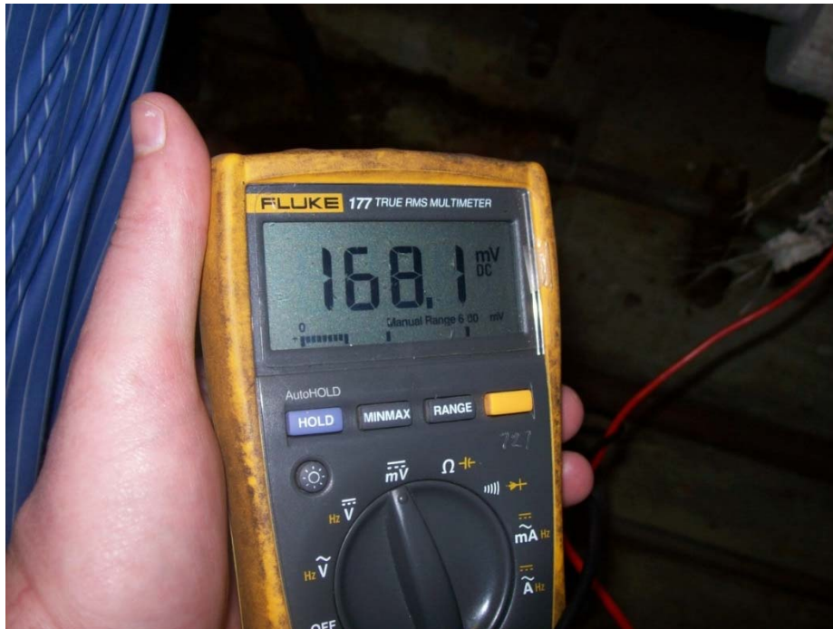
Figure (H1b): A view of the Fluke meter display at 0.168 volts DC, measured from pipe to earth ground.
