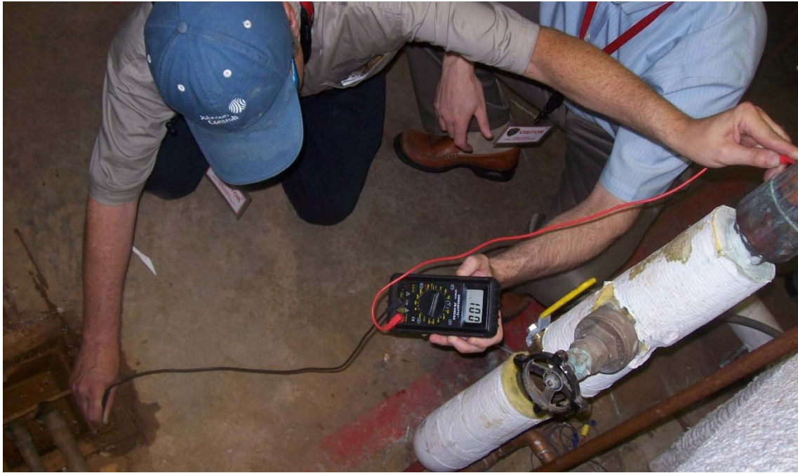
Figure (H3e): A view of DC voltage observed between pipe and floor drain, at Jail #3.
