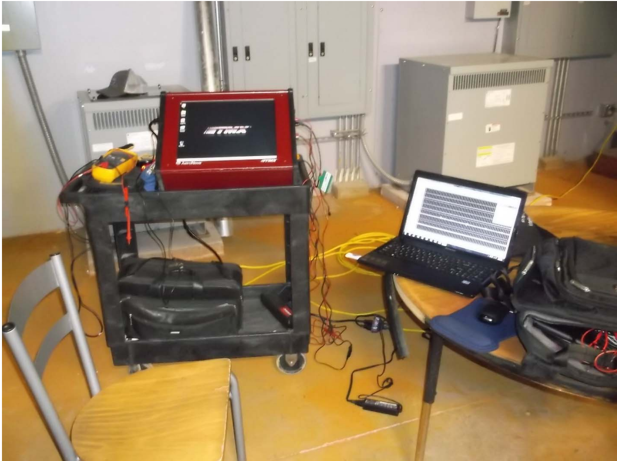
Figure (T1a): A view of the AstroNova testing equipment, set up on site. Initial testing was done with the Omega volt ohm meter. The measurement showed nominal 0.4 volts DC on the HVAC piping system (pipe to earth ground). Follow up electrical testing was done with a high end data logging system (AstroNova). The data logging was done for the HVAC piping system, as well as the plumbing piping system and the fire protection (sprinkler) piping system. Each AstroNova test was done for 3 minutes, collecting 900,000 electrical samples during each 3 minute test (180 seconds per test). This is 5,000 samples per second. For the HVAC piping system, the 3 minute test data indicated 0.409 volts DC. When zoomed in to display only 80 data points, the displayed data was also 0.409 volts DC. For the Plumbing piping system, the 3 minute test data indicated 0.898 volts DC. When zoomed in to display only 80 data points, the displayed data was 1.028 volts DC. For the Fire Protection piping system, the 3 minute test data indicated 0.423 volts DC. When zoomed in to display only 80 data points, the displayed data was 0.432 volts DC.
