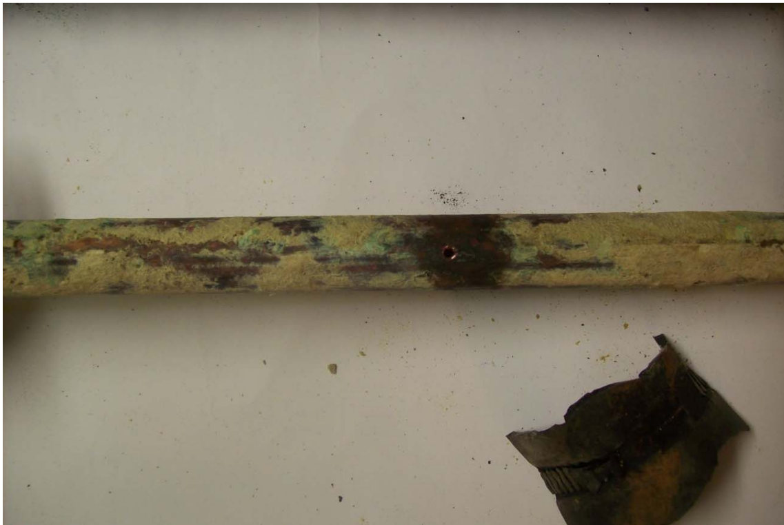
Figure (H2e): A view of the pinhole (when green nodule poked with screwdriver).
