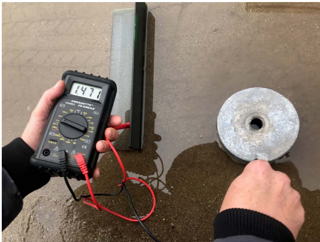
Figure (S1c): A view of a magnesium anode and a section of 2" steel angle iron (in a puddle) in an unpaved parking lot. The Omega volt ohm meter indicates 1.47 volts DC. This is the galvanic potential of magnesium above steel (magnesium at nominal 1.6 volts and rusted steel at nominal 0.13 volts). This magnesium anode is designed to be bolted into a chiller head. In practice the magnesium anode sacrifices to protect the cast iron chiller head.
