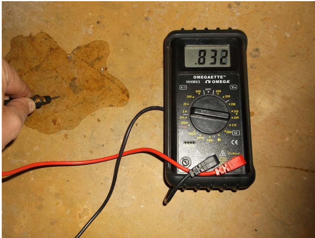
Figure (H4d): A view of DC voltage observed from pipe to wet floor slab.
