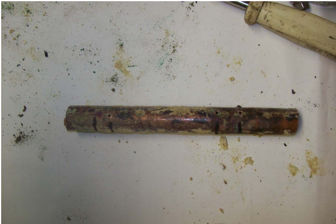
Figure (H2g): A view of a 6 inch section of pipe with 4 pinholes.
