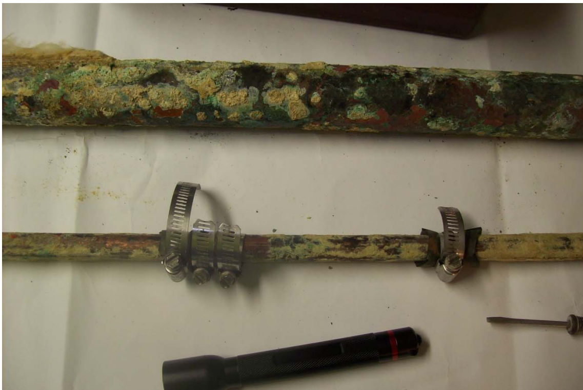
Figure (H2c): A view of removed copper piping with hose clamps in place.
