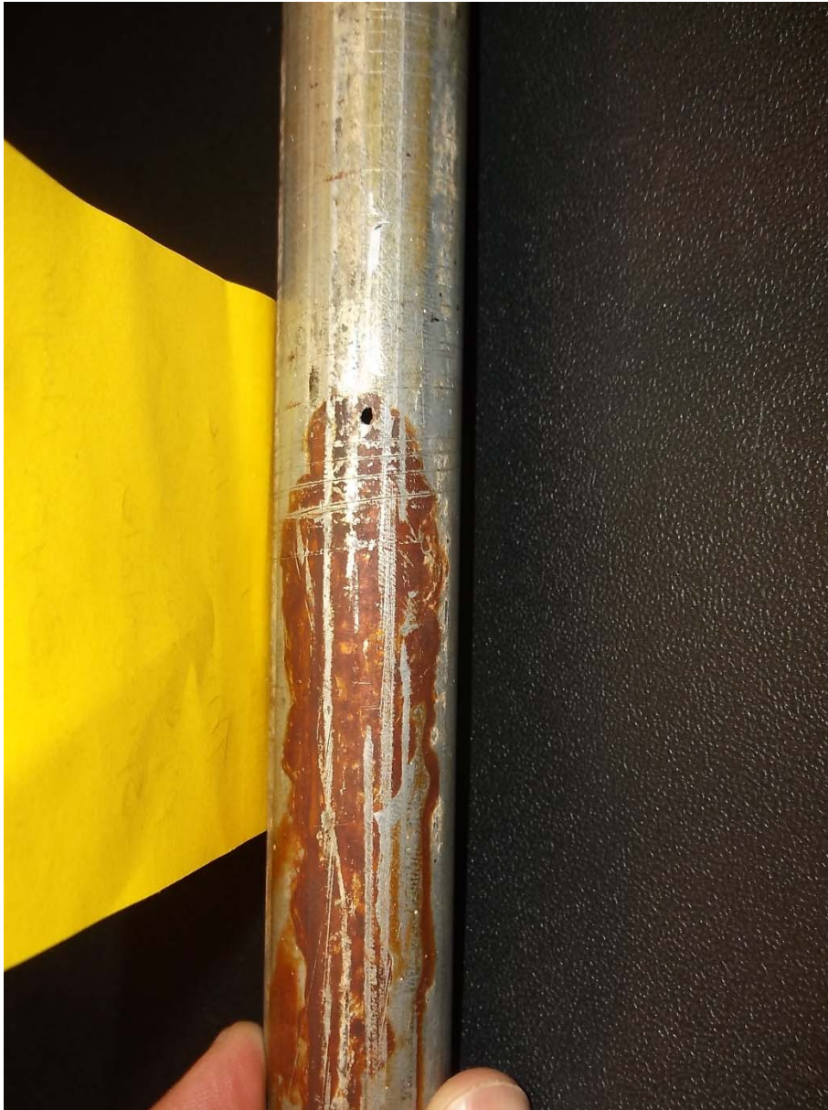
Figure (H4a): A view of a pinhole leak in steel schedule 5 piping. The rust stain is from leaked water. This piping served an HVAC water source heat pump system.
