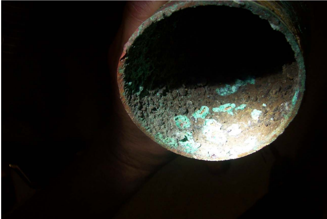
Figure (H3c): An interior view of a failed copper pipe.
