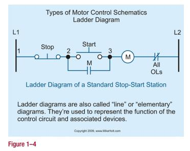
The ladder diagrams in Figures 1–4 and 1–5 illustrates electrical function, showing the M contacts in parallel with the start pushbutton to form what's called a "holding circuit." The physical location of the M contacts isn't shown in the ladder diagram.
